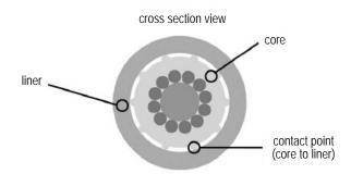
TFXtreme's unique design incorporates a splined core to achieve the "impossible." Ridges of the core allow a close fit with the cable's inner liner, but with minimum contact, so the core glides back and forth smoothly. The result - easy movement and minimum lost motion.
